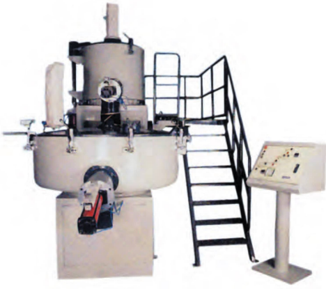
COMPOUNDING MIXER - COOLER
